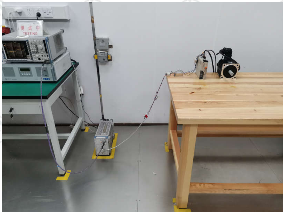
CONDUCTED EMISSION TEST SETUP
